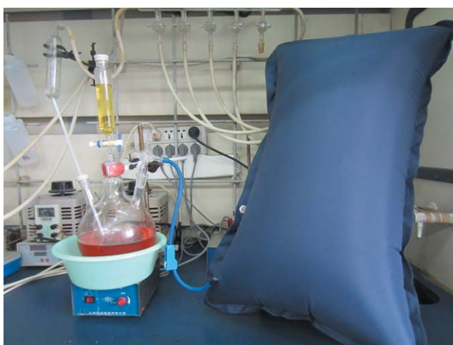
Figure 1 The reaction apparatus used for the aerobic oxidation of propargyl alcohol
