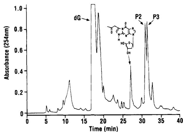
**Figure 4.** HPLC chromatogram (system 1) obtained upon analysis of an incubation mixture of dG and  $\alpha$ -acetoxyNPIP.
