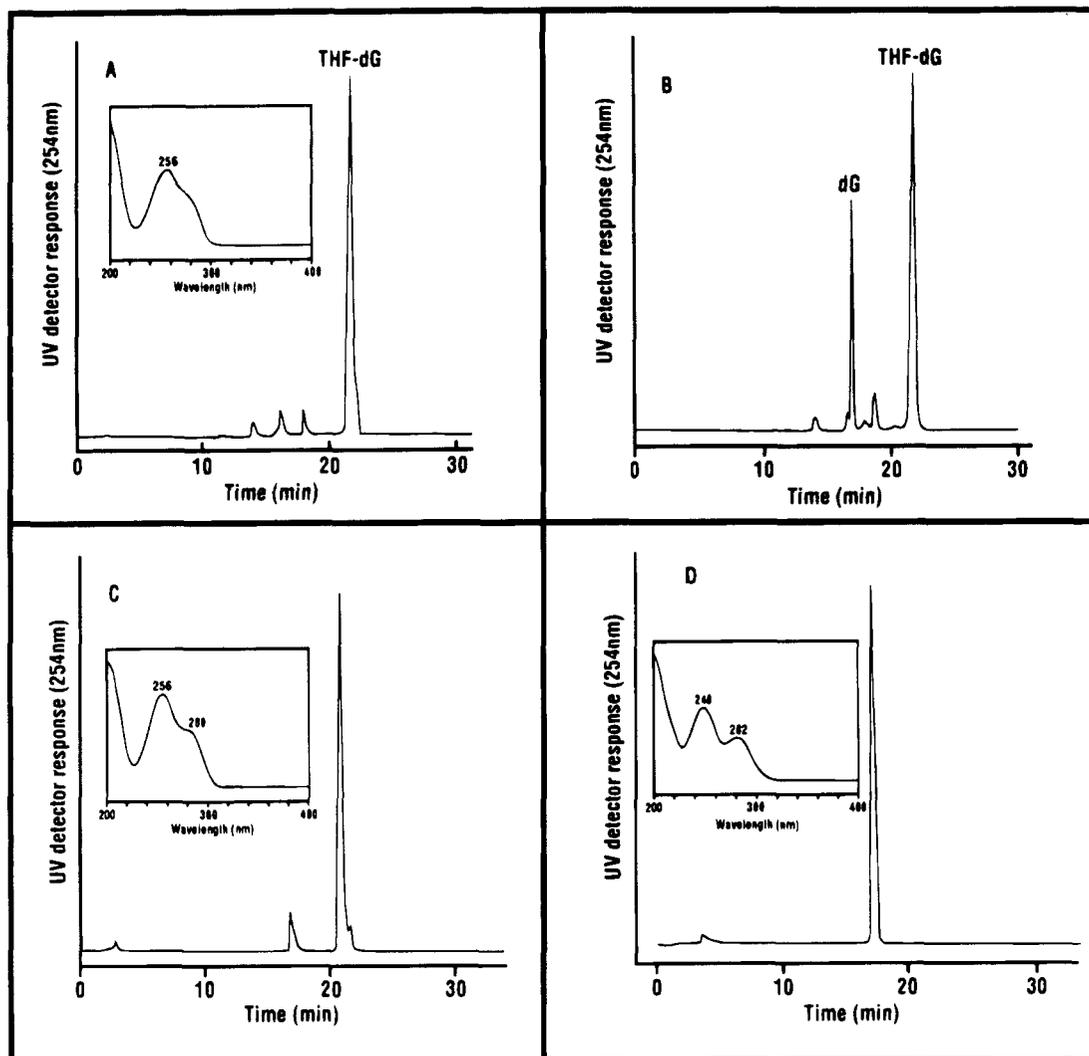
**Figure 7.** HPLC chromatograms (system 5) and UV spectra (insets) of (A) THF-dG synthesized from THF-Cl; (B) a mixture of THF-dG and dG produced by storing THF-dG in pH 7.0 phosphate buffer at  $-20^{\circ}\text{C}$  overnight; (C)  $N^2$ -(4-hydroxybutyl)dG produced by  $\text{NaBH}_4$  treatment of THF-dG; and (D)  $N^2$ -(4-hydroxybutyl)guanine produced by HCl hydrolysis of  $N^2$ -(4-hydroxybutyl)dG.
