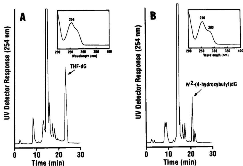
**Figure 10.** HPLC analysis (system 5) of (A) products from reaction of THF-OH with dG, showing formation of THF-dG and its UV spectrum in the inset, and (B) products formed upon treatment of A with NaBH<sub>4</sub>. The UV spectrum of N<sup>2</sup>-(4-hydroxybutyl)dG, formed by reduction of THF-dG, is shown in the inset.
