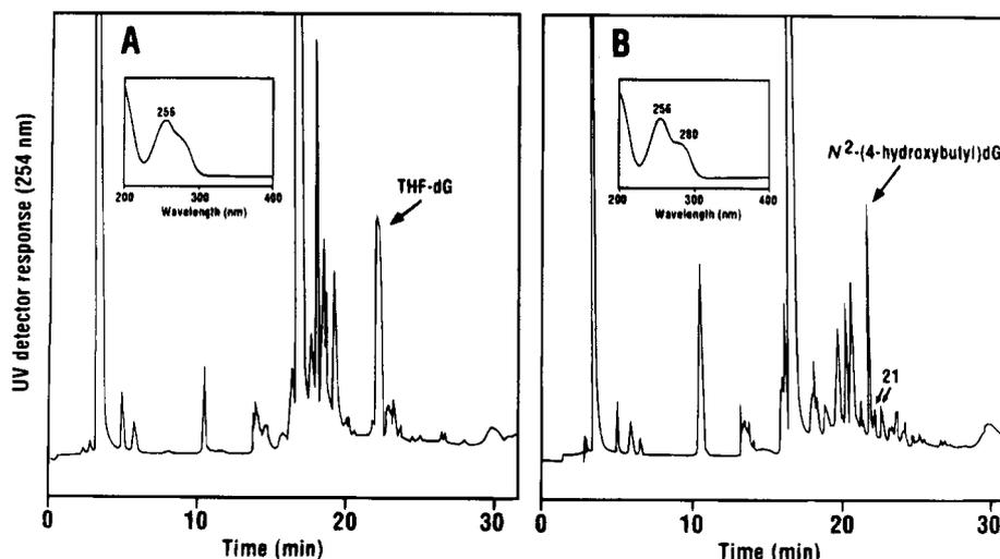
**Figure 9.** HPLC analysis (system 5) of (A) products from reaction of  $\alpha$ -acetoxynPYR with dG, showing formation of THF-dG and its UV spectrum in the inset, and (B) products formed upon treatment of A with  $\text{NaBH}_4$ . Inset is UV spectrum of the peak marked  $N^2$ -(4-hydroxybutyl)dG formed by reduction of THF-dG. Detection of diastereomeric adducts 21 (Figure 3A) is also indicated.
