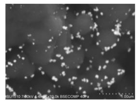
Fig. 4: SEM image of the composite obtained in methanol
