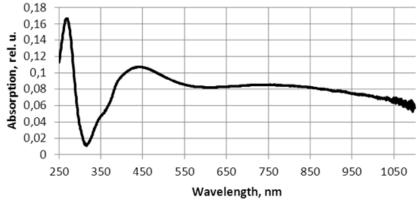
Fig. 2: Plasmon resonance spectrum of colloidal solution of silver nanoparticles prepared from silver palmitate
