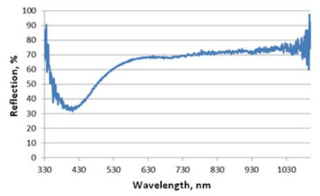
Fig. 6: Diffuse reflection spectrum of the UHMWPE modified by silver nanoparticles
