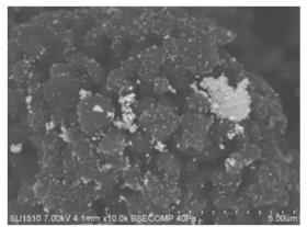
Fig. 5: SEM image of the composite obtained in ethylene glycol
