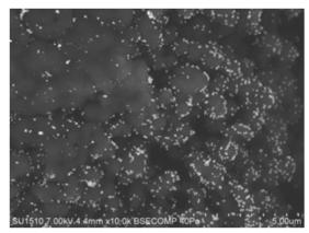
Fig. 3: SEM image of the composite obtained in ethanol
