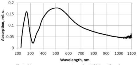
Fig. 1: Plasmon resonance spectrum of colloidal solution of silver nanoparticles prepared from silver laurate
