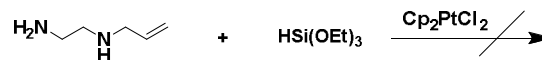
Scheme 2. (Dicyclopentadiene) platinum(II) dichloride catalyst for the hydrosilylation of the diamino chelating alkene with triethoxysilane.
