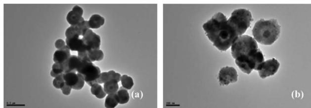
**Fig. 4** TEM images of (a) citrate-capped Au nanoparticles and (b) L-proline-cysteine conjugate-modified Au nanoparticles.
