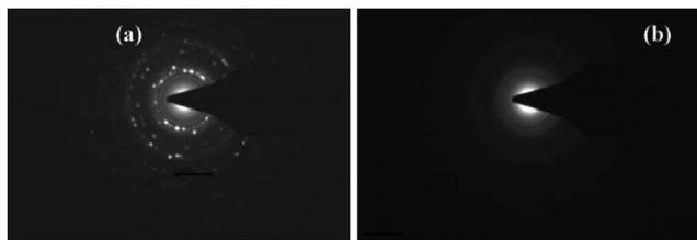
**Fig. 5** Electron diffraction of (a) citrate-capped Au nanoparticles and (b) L-proline–cysteine conjugate on Au nanoparticles.
