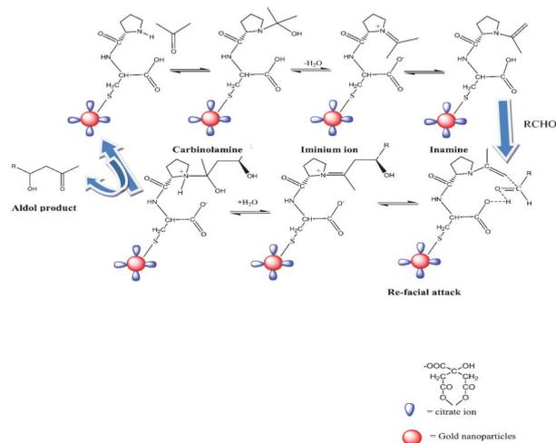
**Scheme 1** Proposed mechanism of the direct aldol reaction catalyzed by L-proline–cysteine conjugate on citrate-capped Au nanoparticles.
