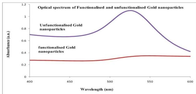
**Fig. 2** UV-Visible analysis of bare Au nanoparticles and L-proline-cysteine conjugate functionalized on Au nanoparticles.
