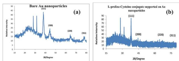
**Fig. 6** (a) X-ray diffraction of citrate-capped Au nanoparticles and (b) L-proline–cysteine conjugate supported on Au nanoparticles.
