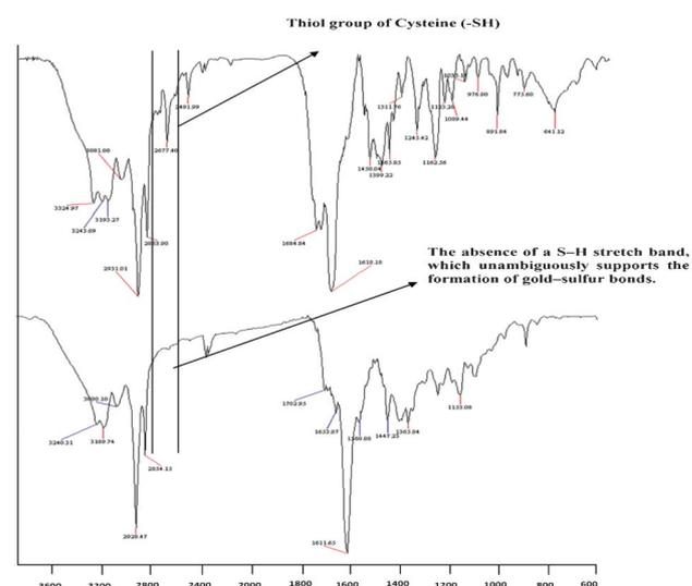
Fig. 1 IR spectra of (a) L-proline–cysteine conjugated product and (b) L-proline–cysteine conjugated product supported on Au nanoparticles (note the disappearance of the S–H stretching).
