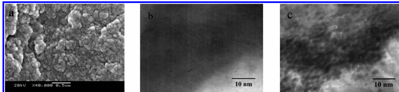
Figure 2. Representative SEM and TEM images of the polymers. (a) 4a-2 (SEM); (b) ionic liquid-soaked Pd(OAc) 2 on 4a-2 (0.53 mmol/g Pd(OAc) 2 loading level) (TEM); and (c) ionic liquid-stabilized Pd nanoparticles on 4a-2 after hydrogenation (TEM).
