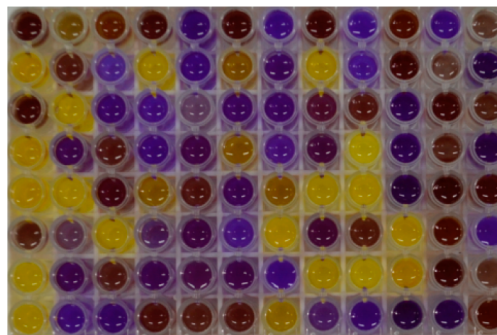
Figure 1. Mutant library screening for the high activity of nitrilases in a 96-well plate.
