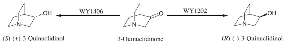
**Scheme 1.** Bioreduction of 3-quinuclidinone to (*S*)- or (*R*)-3-quinuclidinol by isolated microorganisms.
