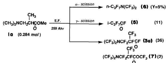
From **1a**, the perfluoromethyl ester **7** is formed in small yield (yield=2%) together with the corresponding perfluoro(3-dimethylamino-isobutyryl fluoride) (**3a**) (yield=36%). From **1** having cyclic amino-substituents, cleaved products arising from  $\alpha$ -scission were the main by-products. A typical example occurs in the fluorination of **1d**.
