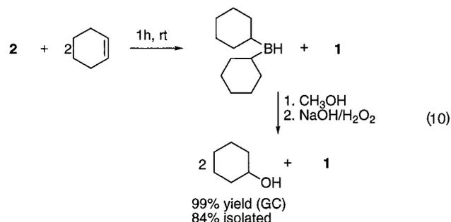
Oxidation of the methanolized solution in THF using alkaline hydrogen peroxide afforded cyclohexanol in quantitative yields (99% by GC), which was also isolated, free of amine by simple acid–base manipulations, in 84% yield.
