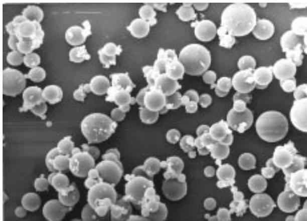
Figure 3. Scanning electron micrograph of the molecularly imprinted polymer beads. The image was obtained using an ISI 100A SEM at 25 kV with a magnification of 1000 $\times$  (reproduced at 60% of original).
