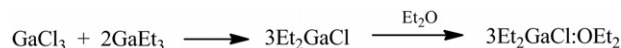
Scheme 5. Generation of Et 2 GaCl from GaEt 3 followed by its complexation with ether.
