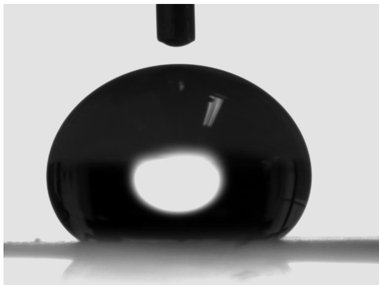
Figure 1. Shape of a water droplet on a glass surface coated with compound 2c ; contact angles are 136.4^\circ and 136.5^\circ , resp.
