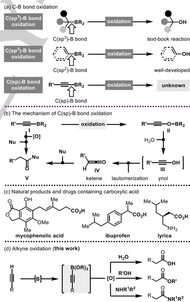
**Figure 1.** (a) C–B Bond Oxidation. (b) C(sp)–B Bond Oxidation Mechanism. (c) Carboxylic Acids in Natural Products and Drugs. (d) Alkyne Oxidation.
