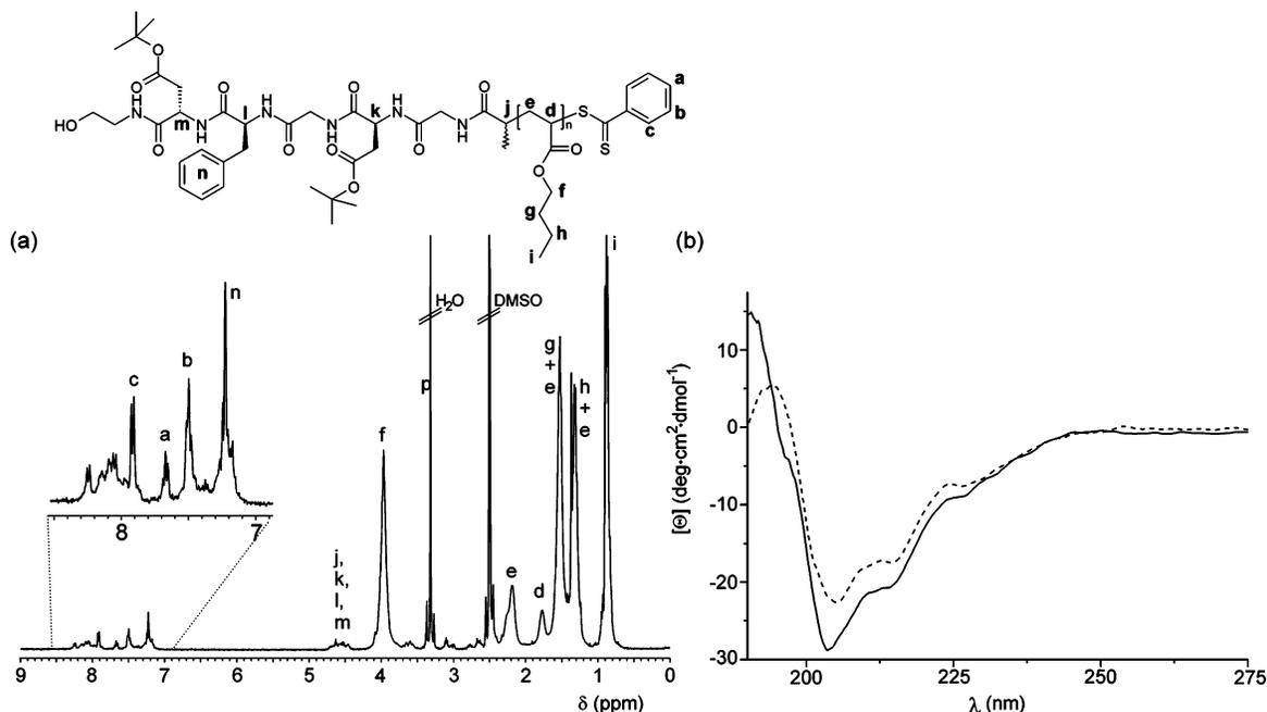
**Figure 5.** (a) <sup>1</sup>H NMR spectrum (DMSO-*d*<sub>6</sub>) of oligopeptide-poly-*n*-butyl acrylate conjugate **6** and (b) CD spectrum of oligopeptide **5** (dashed line) and oligopeptide-poly-*n*-butyl acrylate conjugate **6** (solid line).
