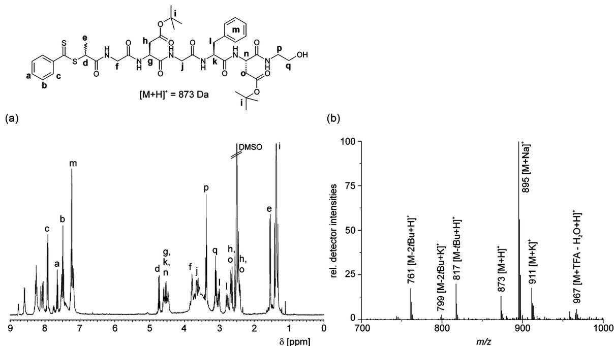
**Figure 3.**  $^1\text{H}$  NMR spectrum ( $\text{DMSO-}d_6$ ) (a) and ESI-MS spectrum of oligopeptide transfer agent **5** (b).
