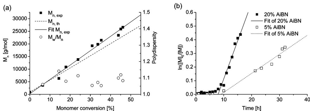
**Figure 4.** RAFT polymerization of *n*BA controlled by **5** at 60 °C: molecular weight ( $M_{n,\text{GPC}}$ ) vs conversion (a) and first-order kinetic plot  $\ln([M]_0/[M])$  vs reaction time (b) (Conditions:  $[n\text{BA}]_0/[5]_0/[AIBN]_0 = 375/1/0.2$ ,  $\text{DMF} = 60 \text{ vol } \%$ .)
