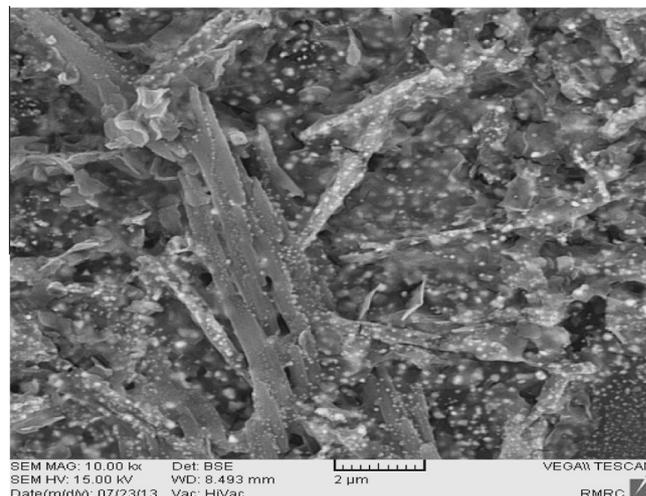
Figure 2. Typical SEM image of samples after deposition of Pd.
