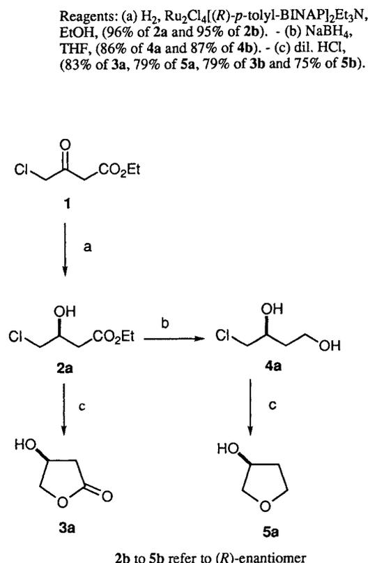
MTPA ester. The synthesis of the (*R*)-enantiomers **3b** (79%) and **5b** (75%) was accomplished from (*R*)-enantiomers **2b** and **4b** under similar reaction conditions. We presume the mechanism of the cyclization reaction to be that depicted in Scheme 2. To the best of our knowledge, these cyclizations of  $\alpha$ -chlorobutanoate **2** and  $\alpha$ -chlorobutanediol **4** have not previously been reported<sup>[9]</sup>.
