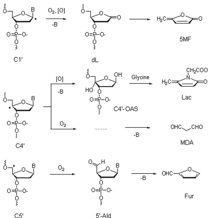
Figure 1. Characteristic end products of oxidative damage to dR analyzed in this study, and the mechanisms of their formation from free radical precursors. Abbreviations dL, C4'-OAS, and 5'-Ald stand for 2-deoxyribose-2-aldose, C4'-oxidized abasic site, and oligonucleotide-5'-aldehyde, respectively.
