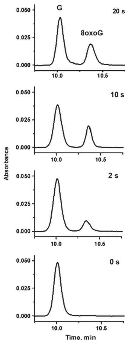
Figure 4. HPLC profiles showing the peaks of G and 8oxoG in the dsDNA/carbonatopentamminecobalt(III) perchlorate system for the first 20 s of exposure to UV light. The products were detected at 305 nm to improve the 8oxoG-to-guanine peak intensity ratio.
