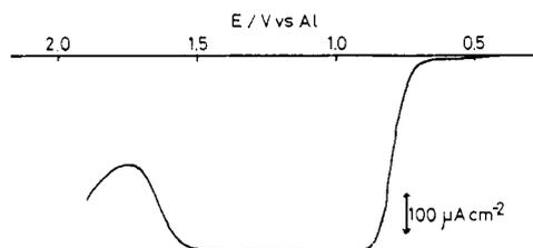
**Figure 3.** Normal pulse voltammogram of  $4.6 \times 10^{-3}$  M TPA in a 1:1:1 melt (pCl = 10.4): sweep rate,  $2 \text{ mV s}^{-1}$ ; pulse length, 48 ms; temperature  $40^\circ \text{C}$ .
