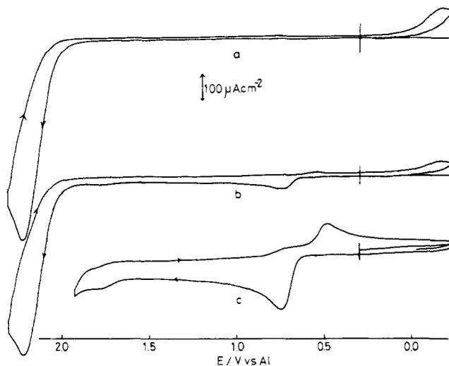
**Figure 6.** Cyclic voltammograms of 1.16 × 10<sup>-2</sup> M DMA at a sweep rate of 100 mV s<sup>-1</sup> and a temperature of 40 °C: (a) melt pCl 8.4; (b) melt pCl 5.8; (c) as (b), but current sensitivity × 5.
