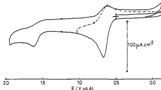
**Figure 7.** Cyclic voltammograms of 1.6 × 10<sup>-3</sup> M DMT in a melt of pCl 5.5 at 40 °C: sweep rate, 100 mV s<sup>-1</sup>.
