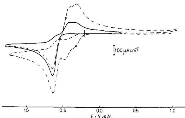
**Figure 5.** Cyclic voltammograms in a 50 vol. % melt-benzene mixture (pCl 3.0) at 40 °C: sweep rate, 100 mV s<sup>-1</sup>; solid line shows the behavior observed for 4.1 × 10<sup>-3</sup> M DMA on the first sweep while the line represented by (---) shows the behavior on the second sweep; the broken line shows the effect of adding TMB to this solution.
