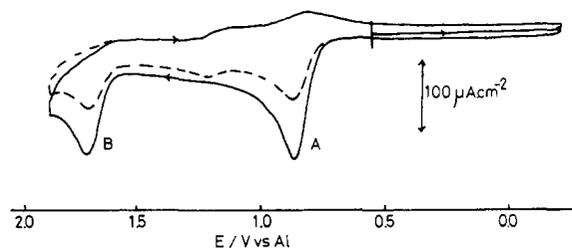
**Figure 1.** Cyclic voltammogram of  $4.6 \times 10^{-3}$  M TPA in a 2:1 melt (pCl 15) at  $40^\circ\text{C}$ : sweep rate,  $100\text{ mV s}^{-1}$ ; solid line, first sweep; broken line, second sweep.
