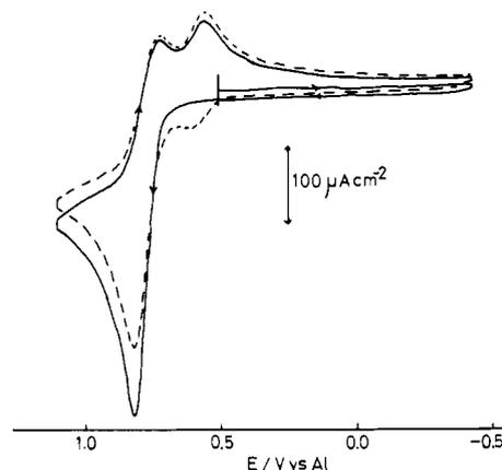
**Figure 4.** Cyclic voltammogram of  $4.2 \times 10^{-3}$  M TPA in a melt of pCl 6.8 at  $40^\circ \text{C}$ : sweep rate,  $100 \text{ mV s}^{-1}$ ; solid line, first sweep; broken line, second sweep.
