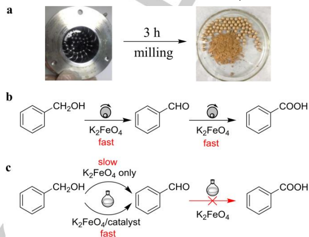
Figure 2. (a) Photos of K_2FeO_4 /benzyl alcohol reaction system before and after ball milling. (b-c) Comparison of K_2FeO_4 oxidation of benzyl alcohol by solvent-free mechanical milling and traditional solvent-based route. [5a]
