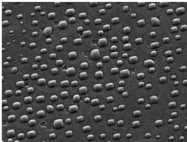
Fig. 4. SEM of Ga on GaAs(100) in pre-coalescence stage growth. Sample G8, annealing time = 7 min.
