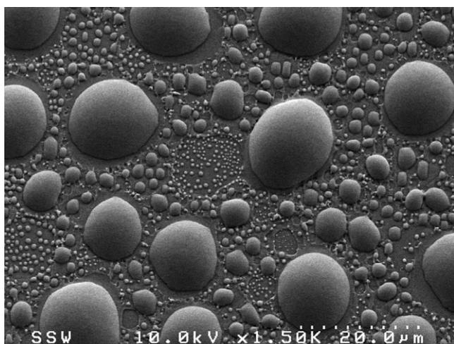
Fig. 6. SEM of Ga on GaAs in coalescence stage growth. Sample G15, annealing time = 5 min.
