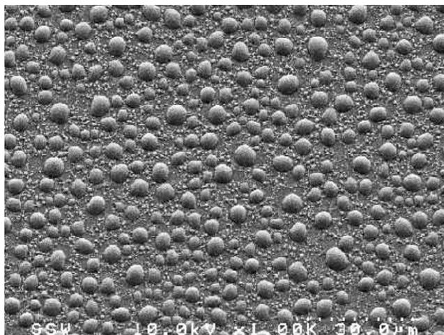
Fig. 5. SEM of Ga on GaAs in early coalescence stage growth. Sample G12, annealing time = 3 min.
