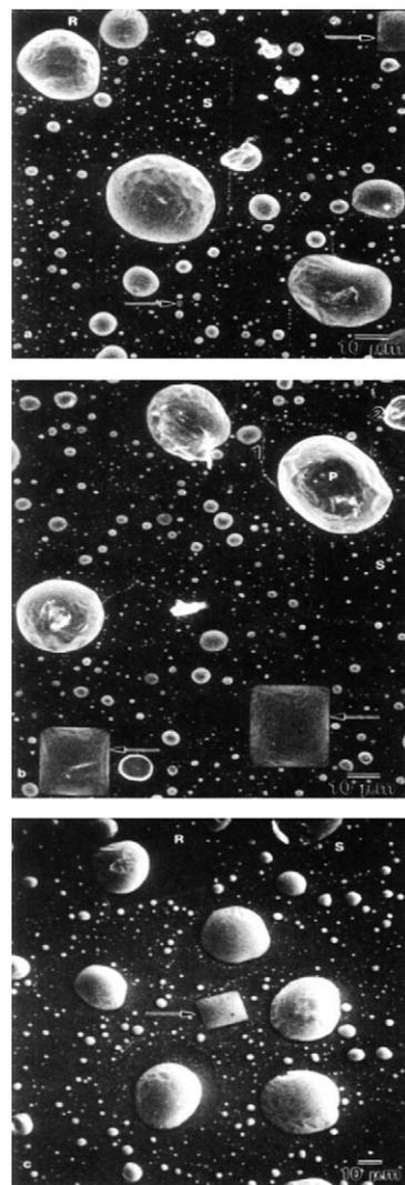
Fig. 10. SEM of In on InP(001) after annealing at 500 °C for 10 min [4]. The three images show two features of the cyclic shape changes. The first feature is that approximately 90% of the clusters are partially spherical with diameters of up to 10  $\mu\text{m}$ . The second feature is that approximately 10% of clusters are associated with rectangular features either in the cluster itself as indicated by the arrows or in the underlying depression as indicated with the R.
