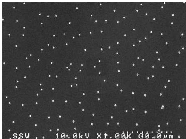
Fig. 2. SEM of Ga on GaAs in pre-coalescence stage growth. Sample G2, annealing time = 5 min.
