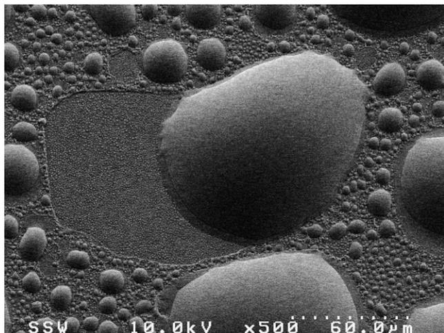
Fig. 9. SEM of Ga on GaAs in cohesive aggregation stage growth. Sample G16, annealing time = 5 min.
