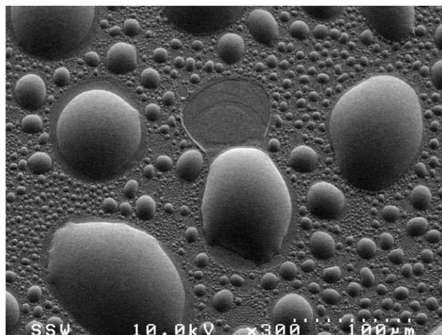
Fig. 7. SEM of Ga on GaAs in cohesive aggregation stage growth. Sample G16, annealing time = 5 min.
