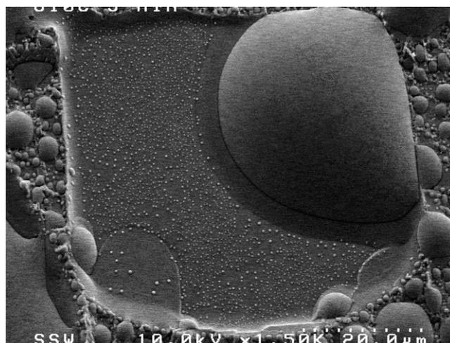
Fig. 8. SEM of Ga on GaAs in cohesive aggregation stage growth. Sample G16, annealing time = 5 min.
