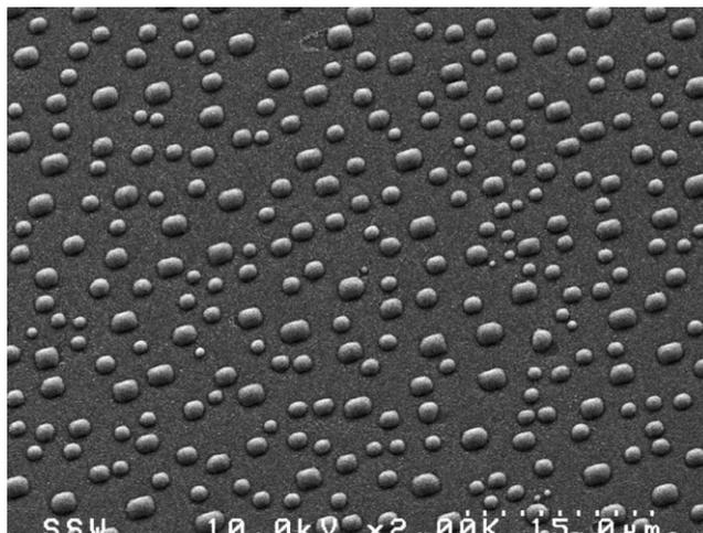
Fig. 3. SEM of Ga on GaAs(100) in pre-coalescence stage growth. Sample G7, annealing time = 7 min.
