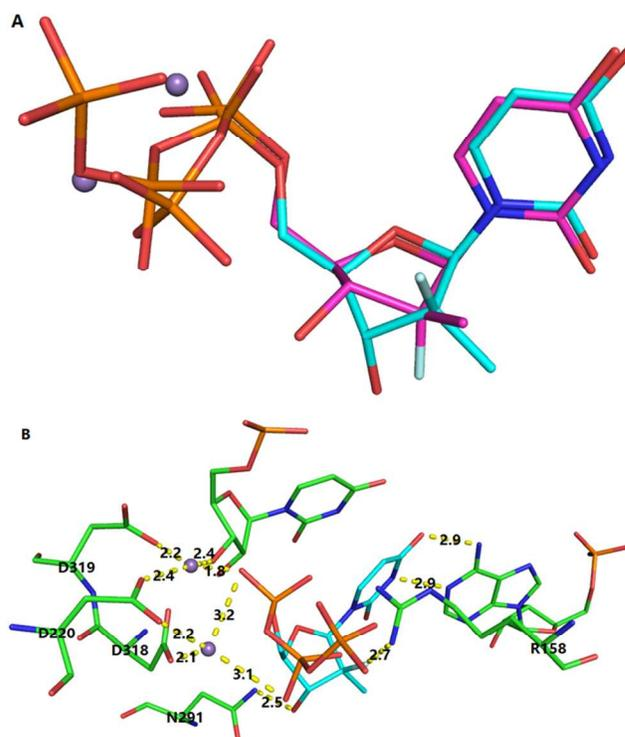
**Figure 5.** Docking models of **23** (cyan) bound to NS5B and co-crystal structure of **24** (magenta)/NS5B (PDB code: 4WTG). (A) **23** and **24** were overlaid to show the differences. (B) Recognition of **23** by NS5B.
