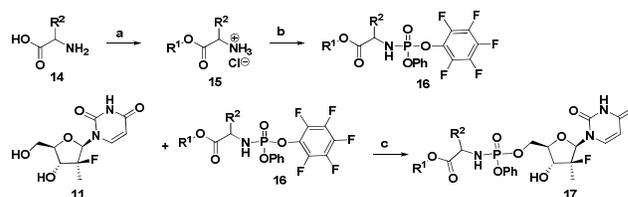
Reagents and conditions: a) SOCl<sub>2</sub>, alcohol, reflux, 2 h - 24 h, 75% - 95%; b) phenyl dichlorophosphate, Et<sub>3</sub>N, 2,3,4,5,6-pentafluoro phenol, DCM -78 ° C - rt, 4 h, 60% - 85%; c) *t*-BuMgCl, THF, 0 ° C, 12 h, 28% - 35%.
