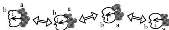
Figure 6. Schematic illustration of the cooperative plating of the copper particles. i, current density; a, cathodic site; b, anodic site;
