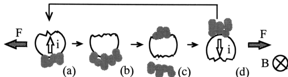
Figure 5. Schematic illustration of the reverse mechanism of the moving direction. B, magnetic flux density; i, current density; F, Lorentz force; (a), Initially, silver dendrites deposit at the bottom side.; (b), Because of depletion of silver ions, deposition rate decreases, and motion finally ceases.; (c), Reduction of silver ions starts at the top side which abounds in silver ions. As the dissolution of the substrate at the bottom progresses, the silver dendrites begin to fall off.; (d), At the top side, silver deposition proceeds, and the particle moves in the direction opposite to (a).
