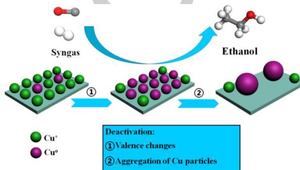
**Fig. 6.** Schematic representation of the deactivation of Cu/SiO<sub>2</sub> catalyst
