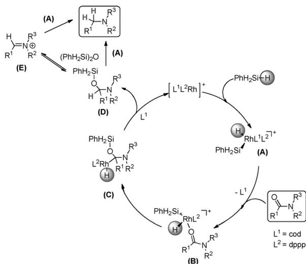
**Scheme 3.** Proposed catalytic cycle for the rhodium-catalyzed hydrosilylation of tertiary amide bonds. The ligands on the rhodium center are named L<sup>1</sup>L<sup>2</sup> for clarity.
