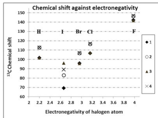
**Figure 4.**  $^{13}\text{C}$  chemical shift of halogenated 5-C plotted against electronegativity of the halogen atom. The electronegativity is 3.98 (F), 3.16 (Cl), 2.96 (Br) or 2.66 (I), respectively, and each of them is higher than that of H atom (2.2). However, the  $^{13}\text{C}$  chemical shifts of the 5-carbons bearing bromo (Br) or iodo (I) atom are lower than those of the carbons bearing H atom in all the nucleosides (**1-4**).
