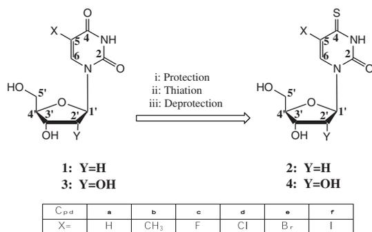
**Scheme 1. Transformation of 5-substituted nucleosides to their 4-thio-analogues.** The starting materials **1** (Y = H) and **3** (Y = OH) were converted to 4-thioanalogues **2** (Y = H) and **4** (Y = OH) via a three reaction process: protection of the OH groups of the sugar moiety, replacement of the oxygen atom at 4-position with a sulfur atom, then removal of the protecting groups on the sugar. X at 5-position represents an H atom, CH<sub>3</sub> (methyl group) or any of the halogens.
