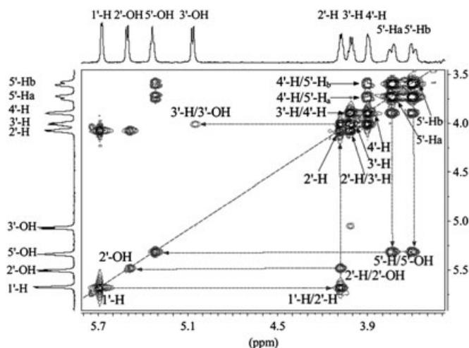
**Figure 1. The sugar section of H-H COSY spectrum of **4e** (5-bromo-4-thiouridine).** Peaks on the diagonal line are the NMR signals of the protons on the sugar. The off-diagonal peaks (cross-peaks) directly correlate the coupled protons. The arrows indicate routes to the coupled partners.
