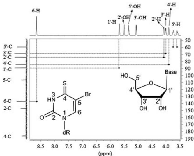
**Figure 2.** H-C COSY spectra of **4e** (5-bromo-4-thiouridine).  $^1H$  NMR is shown at the top.  $^{13}C$  NMR is shown in the left side. Inserts are chemical structures of the sugar and base.
