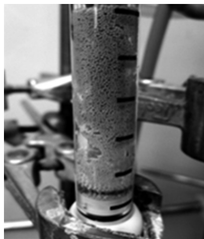
Figure 4. Thiosulfate beads mixed with Celite® for the removal of excess iodine.
