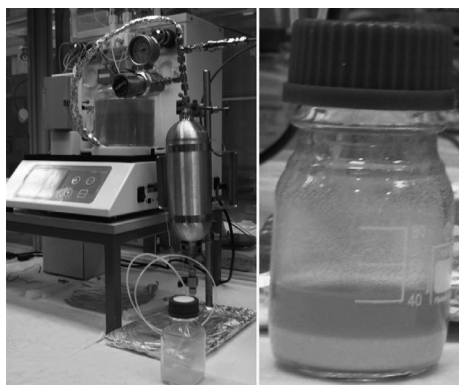
Figure 6. Uniqsis Flowsyn connected to our in-house “pressure chamber”.
