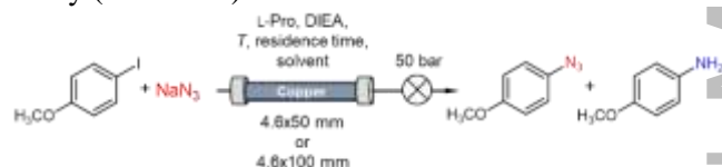
Scheme 3. Copper-catalyzed nitrogenation of 4-iodoanisole with NaN 3 as nitrogen source in a continuous-flow reactor.
