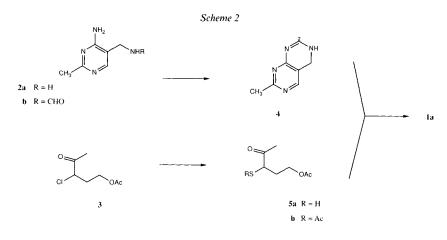
First experiments were performed using the acetate **5b**, easily obtained in over 80% yield by reaction of chloro-acetate **3** with potassium thioacetate in MeOH.
