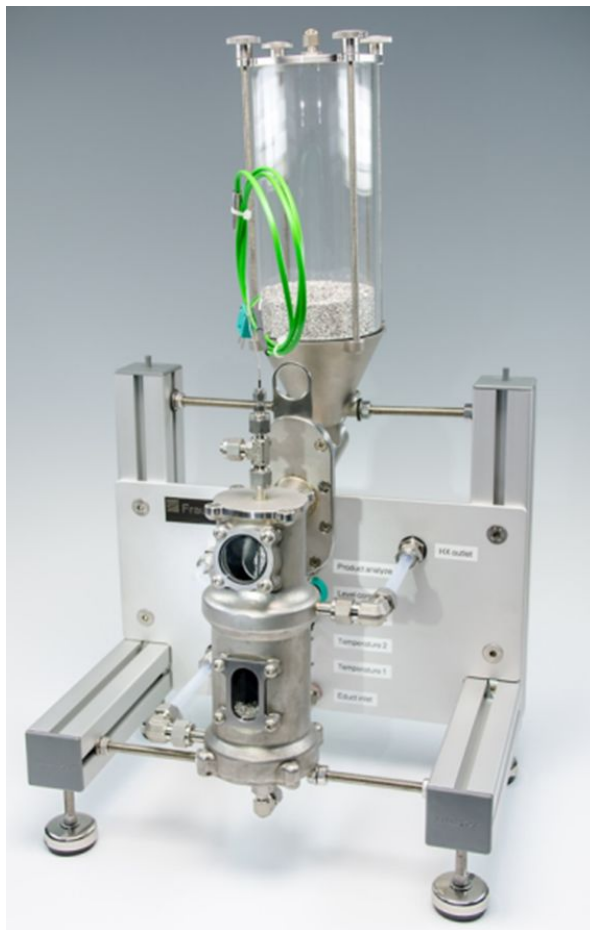
40 Figure 6: Pilot-scale Grignard reagent formation reactor with implemented automated Mg 41 refilling. 42 43 44
