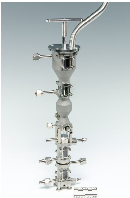
Figure 4: Laboratory-scale Grignard reagent formation reactor including the Mg refilling unit.
