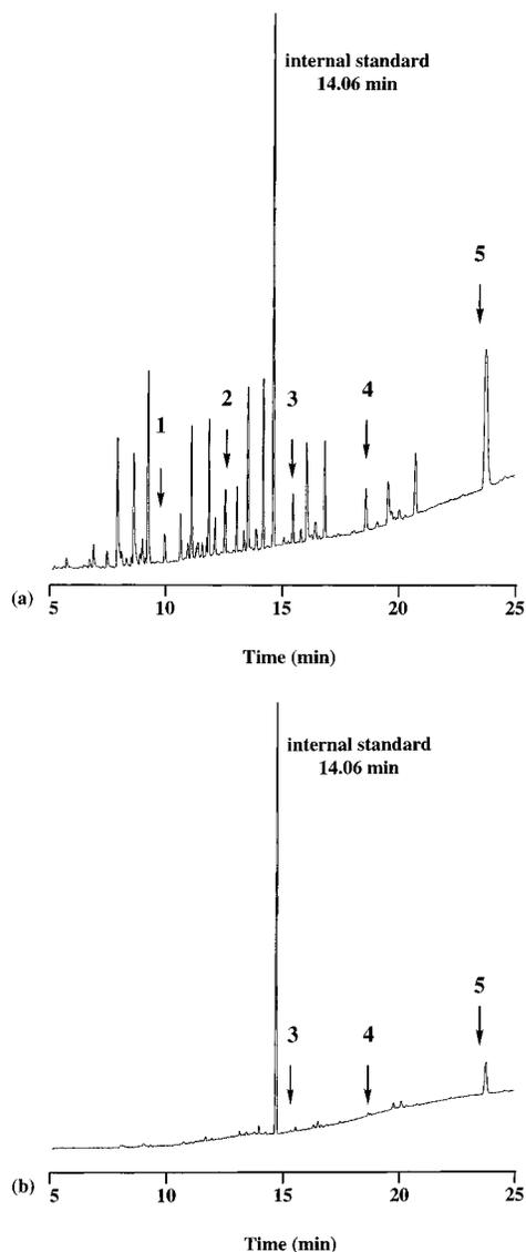
**Figure 2**—GC chromatograms showing separation of the oxidation products detected in the alcohol ethoxylate  $C_{12}E_5OH$ , at air exposure: (a) sample 2, handled at room temperature for 4.5 months; (b) a sample from a newly opened ampule. The peaks are assigned with the numbers corresponding to the identified compounds (1–5). Methyl stearate was used as internal standard.
