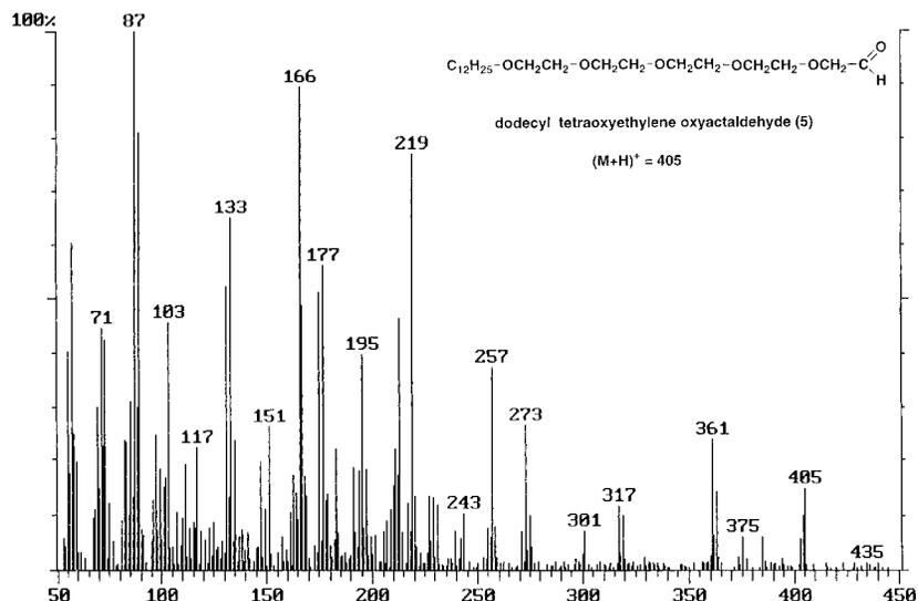
Figure 1—MS—PCI spectrum showing the fragmentation pattern of **5** introduced into the ion source via the direct insertion probe.
