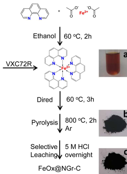
Figure 2. Schematic illustration for the preparation of the FeO x @NGr-C. (a) Photograph of the Fe-phen complex. (b) Photograph of the catalyst precursor before pyrolysis. (c) Photograph of the obtained FeO x @NGr-C.
