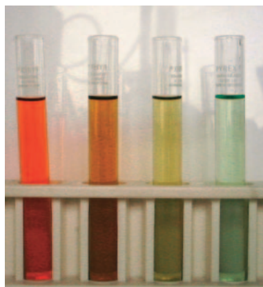
Fig. 9. [\text{Ni}(\text{bzac})(\text{tmen})(\text{H}_2\text{O})_2]\text{I} \cdot 2\text{H}_2\text{O} in 4 different organic solvents, namely nitromethane (NM), 1,2-dichloroethane (DCE), acetone (ACO), and dimethylsulfoxide (DMSO) (from the left).
