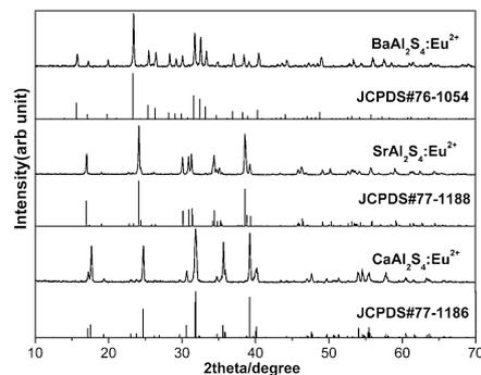
Figure 1. XRD patterns of MAI<sub>2</sub>S<sub>4</sub>:Eu<sup>2+</sup> (M = Ca, Sr, and Ba).
