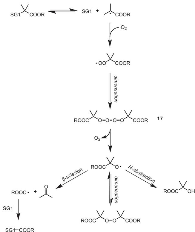
Scheme 5. Proposed mechanism for the formation of the side-product SG1-COOR.
