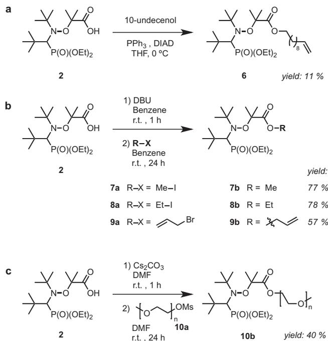
**Scheme 3.** Direct esterification of alkoxyamine **2** by (a) Mitsunobu reaction, (b) nucleophilic substitution of alkyl halides, (c) application to polymer grafting.
