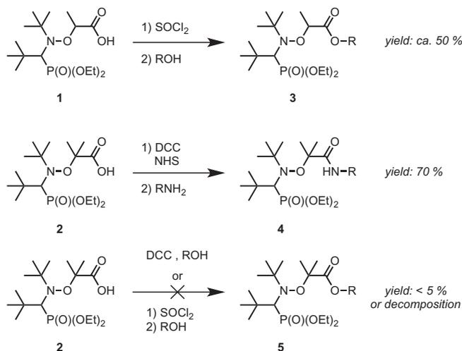
**Scheme 2.** Functionalization of alkoxyamines **1** and **2** by esterification and amidification, respectively.
