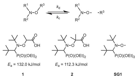
**Scheme 1.** Homolysis of alkoxyamines and structures of labile alkoxyamines **1** and **2** (Ea: activation energy).
