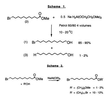
Red-Al<sup>®</sup>) as a 70% solution in toluene does not react rapidly with oxygen and is non-pyrophoric. It has been shown to reduce carboxylic acids and esters,<sup>5</sup> but can also reduce alkyl bromides.<sup>6</sup> It was decided to investigate if Vitride<sup>®</sup> could effect a selective reduction of the carbonyl group in 11-bromoundecanoic acid and the corresponding methyl ester (2).
