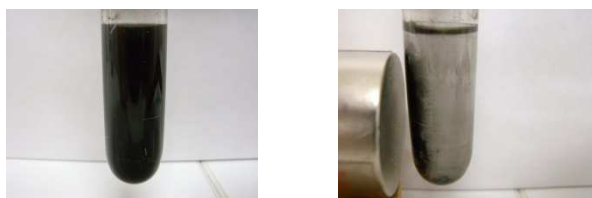
Figure 2. The aerobic oxidation of 2-octanol ( 2a ) in water with Co-Pd alloy nanoparticles 1a . Left: the mixture after the reaction. Right: separation of the Co-Pd alloy nanoparticles from the reaction mixture with a Nd magnet. The recovery of magnetic catalysts took 10–15 min.
