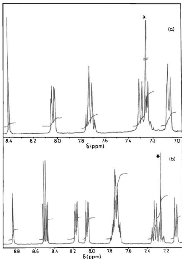
Fig. 2. <sup>1</sup>H NMR of (a) **3** and (b) **6** recorded in CDCl<sub>3</sub>.
