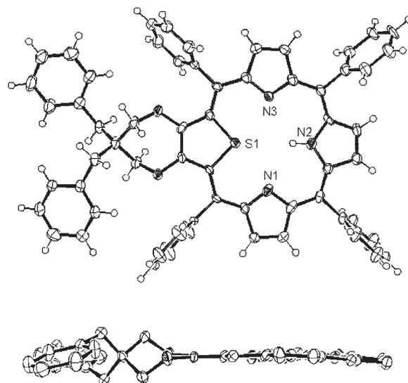
Fig. 4. ORTEP drawing for **6** (top, plane view; bottom, side view). Crystal data: C<sub>64.5</sub>H<sub>49</sub>N<sub>3</sub>O<sub>2</sub>S, purple needles, triclinic, space group = *P*1, *a* = 9.6630(11), *b* = 14.6111(16), *c* = 18.876(2) Å, *V* = 2438.1(5) Å<sup>3</sup>, *Z* = 2, density = 1.2667 g/cm<sup>3</sup>, *T* = 293(2) K, *F*(000) = 978, *R* = 0.0691, *wR*2 = 0.2417.
