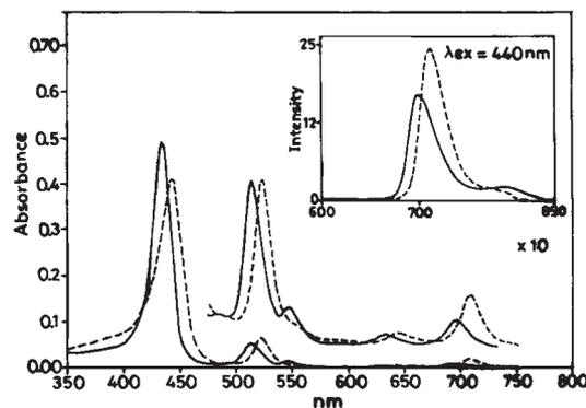
Fig. 3. Absorption and emission (inset) spectra, recorded in toluene, for S<sub>2</sub>TPP (—) and **3** (---).Table 2. Fluorescence Data of  $\beta$ -Thiophene Substituted Porphyrins 1–6 in Toluene
