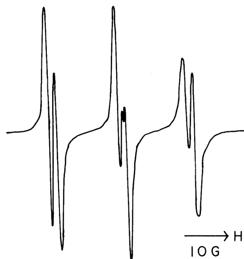
Fig. 2: ESR spectrum of \gamma -irradiated linoleic acid in the ethanol solution containing MNP. Conditions of ESR observation were as follows: gain amplitude, 2,000; modulation width, 0.25 G; response time, 0.3 s; microwave power, 3mW; and sweep rate of magnetic field, 100 G/ 8 min.
