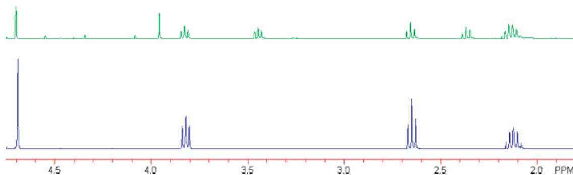
Figure 1. ^1\text{NMR} (400 MHz) spectra at pD = 3.0 (bottom) and pD = 12.7 (top). Bottom signals: 4.70 ppm -CO-CH 2 -O compound 3 , 3.82 ppm, -CH 2 N- compound 3 , 2.65, -CH 2 -CO compound 3 , 2.14 ppm, -CH 2 -CH 2 -CH 2 - compound 3 . Top signals: 4.70 ppm -CO-CH 2 -O compound 3 , 4.55 ppm, -CO-CH 2 -O Cyclol 4.35 -CO-CH 2 -O, Macrocycle, 4.08 -CO-CH 2 -O, NBA, 3.96 ppm -CH 2 - glycolic acid (conjugate base), 3.82 ppm, -CH 2 N- compound 3 , 3.45 -CH 2 N- 2-pyrrolidone, 2.65, -CH 2 -CO compound 3 , 2.36 , ppm -CH 2 -CO 2-pyrrolidone and 2.14 ppm, -CH 2 -CH 2 -CH 2 - compound 3 and 2-pyrrolidone
