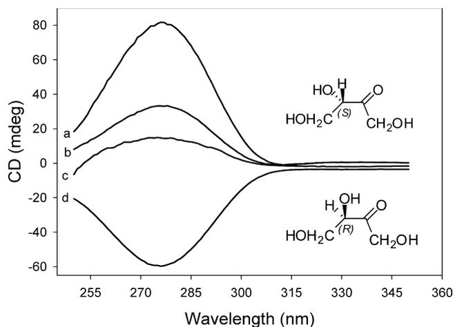
Fig. 8. CD spectra of 1,3,4-trihydroxy-2-butanone produced by parental PDHc-E1 and its E636A and E636Q variants and the E477Q YPDC variant. (a) PDHc-E1 E636Q +  $\beta$ -hydroxypyruvate and glycolaldehyde, (b) PDHc-E1 E636A +  $\beta$ -hydroxypyruvate and glycolaldehyde, (c) PDHc-E1 +  $\beta$ -hydroxypyruvate, and (d) YPDC E477Q +  $\beta$ -hydroxypyruvate and glycolaldehyde. ( $\lambda_{\text{max}} = 278$  nm). Conditions are described under Section 2.
