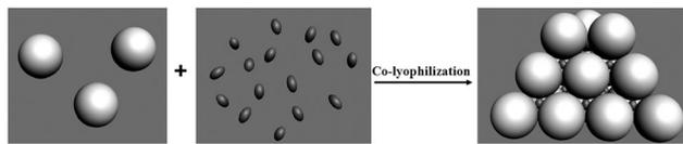
**Fig. 1** The new immobilization method for encapsulating  $\beta$ -gal in the aggregated silica nanoparticles. The gray sphere and the black ellipsoid represent the silica nanoparticles and  $\beta$ -gal, respectively.
