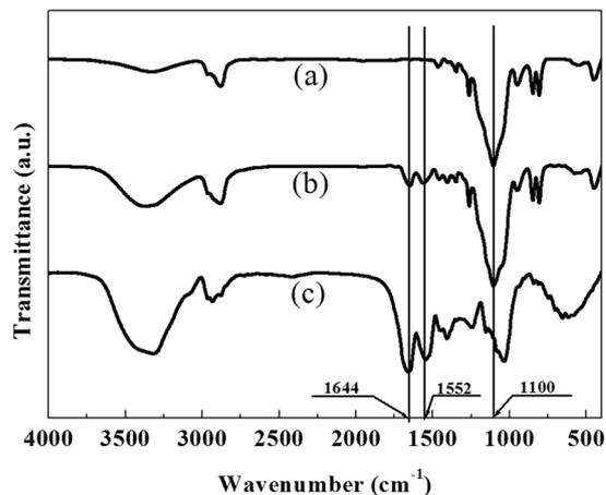
**Fig. 3** FTIR spectrum of: (a) the aggregated silica nanoparticles, (b) the aggregated silica nanoparticles loaded with  $\beta$ -gal, and (c) pure  $\beta$ -gal.
