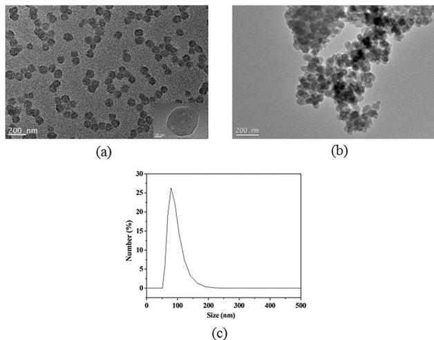
**Fig. 2** (a) TEM images of the silica nanoparticles. Inset: individual silica nanoparticle. (b) The matrix loaded with  $\beta$ -gal. (c) Light scattering measurement of the silica nanoparticles.
