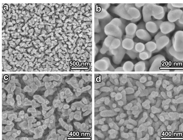
**Figure 1.** Scanning electron microscopy (SEM) images of a)  $\text{Fe}_2\text{O}_3$ , b)  $\text{C-Fe}_2\text{O}_3$ , c)  $\text{Co}_3\text{O}_4\text{-Fe}_2\text{O}_3$ , and d)  $\text{C/Co}_3\text{O}_4\text{-Fe}_2\text{O}_3$  photoanodes.
