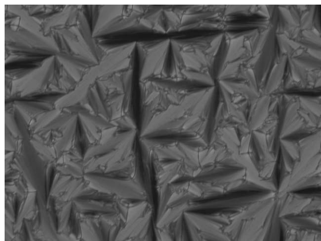
Fig. 3 Polarized optical microscope picture of the liquid-crystalline texture of the oligothiophene 1 at 100\text{ }^{\circ}\text{C} taken during the cooling process.
