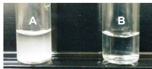
FIGURE 1. Solubility of equimolar concentrations of CuI (A) and bis[(tetrabutylammonium) di-μ-iodo-diiododicuprate(I)] complex (B) in H 2 O.
