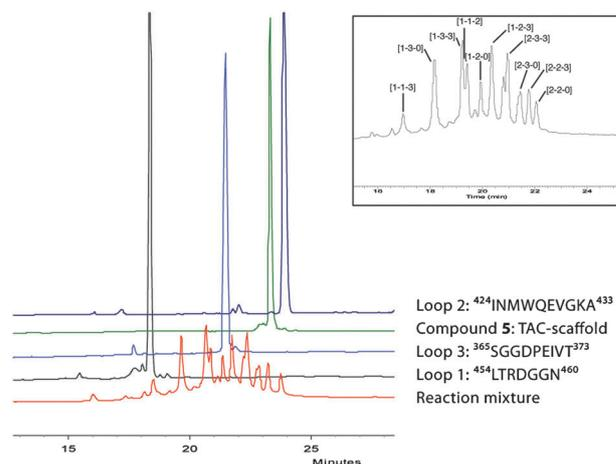
**Fig. 2** HPLC-chromatogram of cyclic azidopeptides containing the conserved epitopes, TAC-scaffold **5** and reaction products of the CuAAC reaction depicted in Scheme 1.
