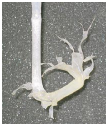
Figure 5. Single-ended 9-mm o.d. Teflon-FEP ampule, used for recording the Raman spectrum, after explosion of less than 500 mg of \text{N}_5^+[\text{P}(\text{N}_3)_6]^- .
