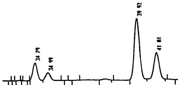
**Figure 1.** Chiral GC resolution on a Cyclodex B column of nonracemic mixtures of cyclopentenes **2-c** and **2-t** from a thermal isomerization of (1*S*,2*R*)-**1**.
