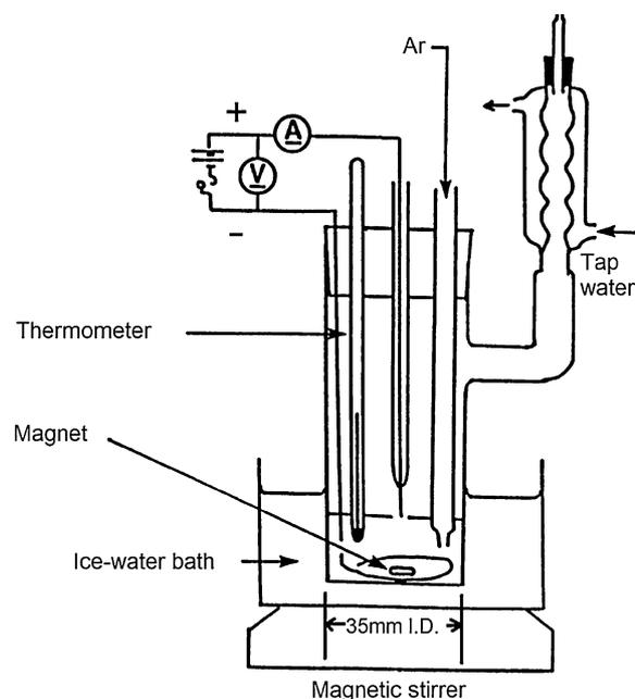
**Figure 3.** Apparatus used for Harada discharge.
