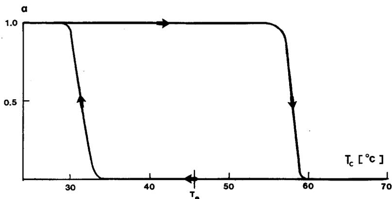
Fig. 3. A typical thermogram for a dehydration/rehydration cycle of a cycled sample under isobaric conditions ( $p_c = 25$  torr). Temperature range, 30–60°C; scanning rate, 3°C h<sup>-1</sup>, particle size, 100–125 μm.  $T_e = 45.7^\circ\text{C}$  refers to the equilibrium temperature from ref. 18.
