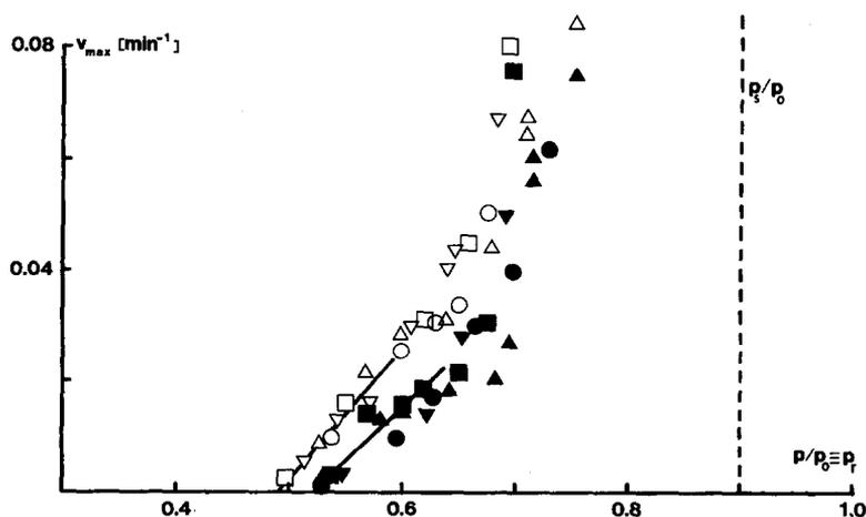
Fig. 8. Maximum reaction rate vs. relative pressure ( $p_r$ ) for the rehydration reaction. Particle size, cf. Fig. 4.  $p_s$  and  $p_0$  refer to the vapour pressures of a saturated barium chloride solution (with respect to  $\text{BaCl}_2 \cdot 2\text{H}_2\text{O}$ ) and of pure water (saturation), respectively.
