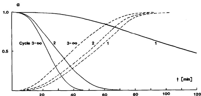
Fig. 1. Dehydration and rehydration progress curves during successive cycles of the reaction  $\text{BaCl}_2 \cdot \text{H}_2\text{O}(s) + \text{H}_2\text{O}(g) \rightleftharpoons \text{BaCl}_2 \cdot 2\text{H}_2\text{O}(s)$
