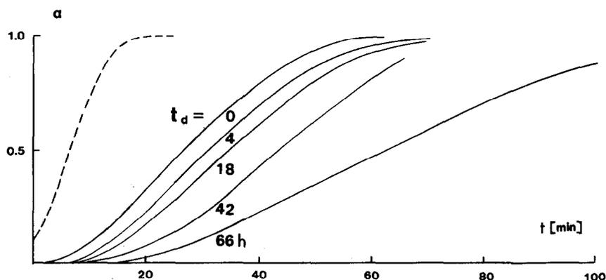
Fig. 2. Rehydration curves for reaction (1) at (48.5 torr,  $44.5^\circ\text{C}$ ). Full curves refer to the rehydration following a complete dehydration (< 99%), after different delay times. The dashed curve was recorded immediately after a 90% dehydration.
