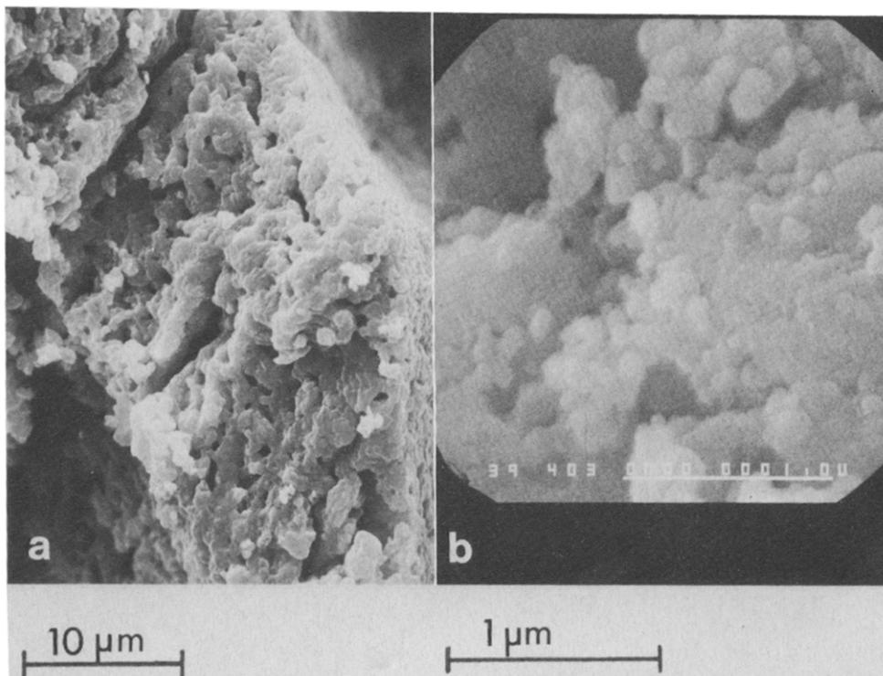
Fig. 6. Scanning electron micrographs showing the internal structure of (a) a sectioned  $\text{BaCl}_2 \cdot 2 \text{H}_2\text{O}$  particle ( $3000\times$ ); (b) a sectioned  $\text{BaCl}_2 \cdot \text{H}_2\text{O}$  particle ( $40000\times$ ).
